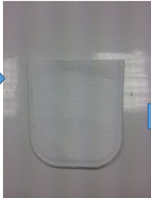
Nylon bags Pore size 25 \mu\text{m}
